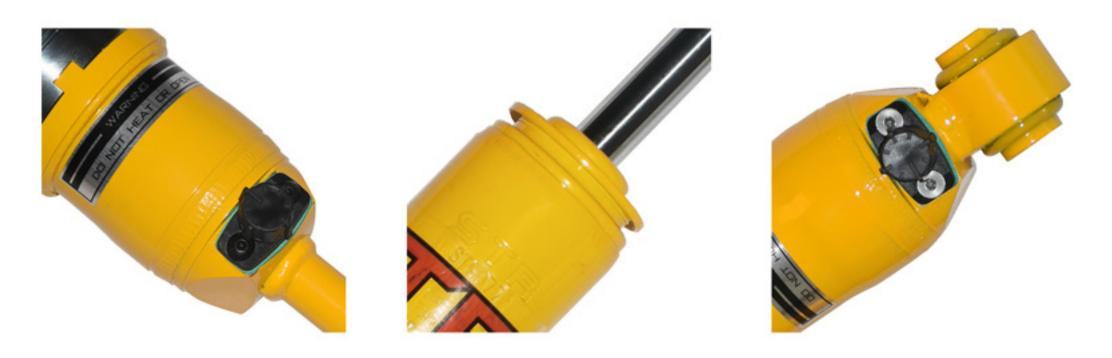
Clockwise direction turn to increasing damp Anti-clockwise direction turn to decreasing damp
