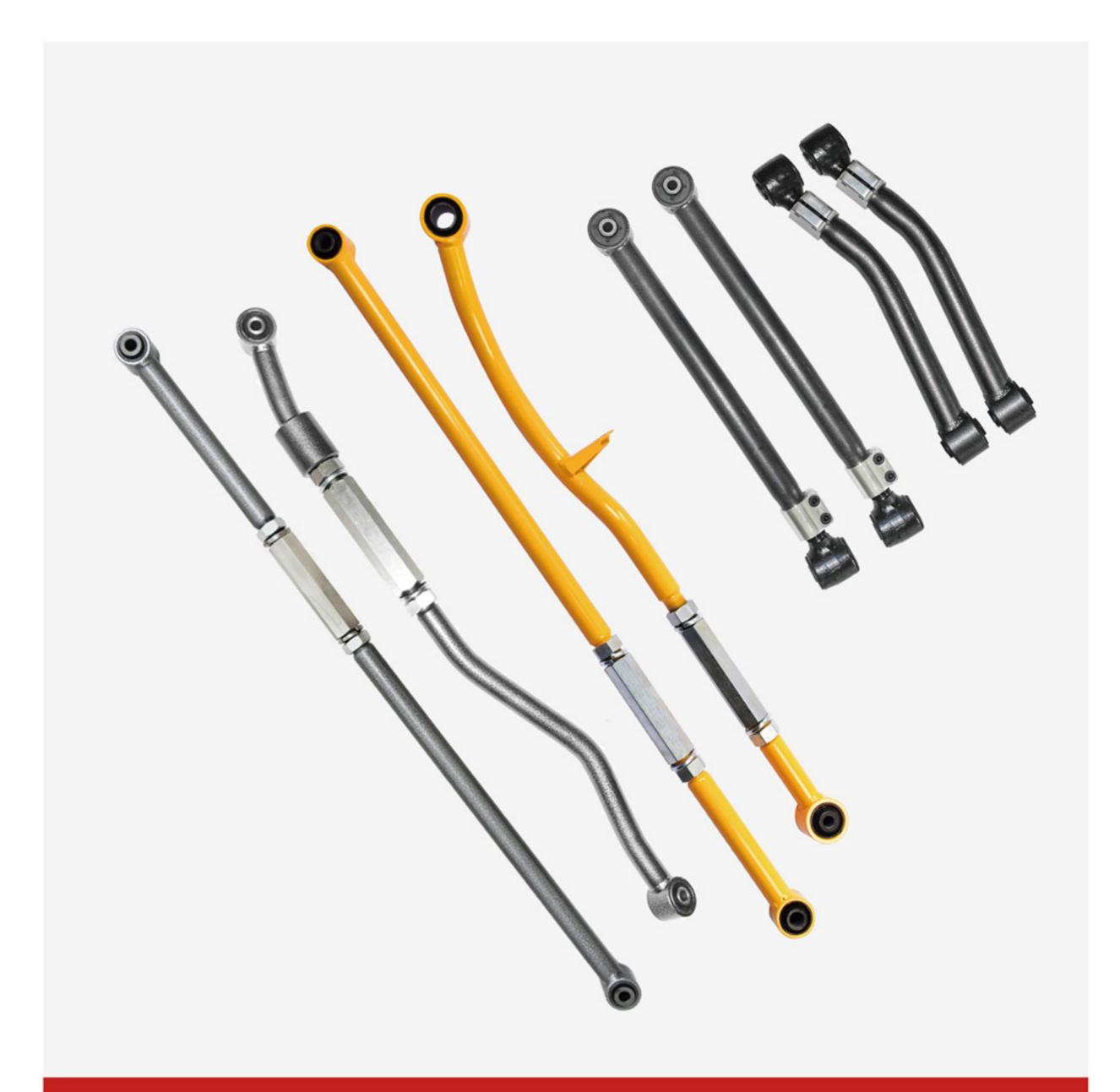
The stop rod is connected between the beams and the rear bridge to ensure that the rear bridge and the front bridge are basically remained in a central axis. The role is to improve the stability of the car, and it can also be understood as a reduction of left -right swing.
